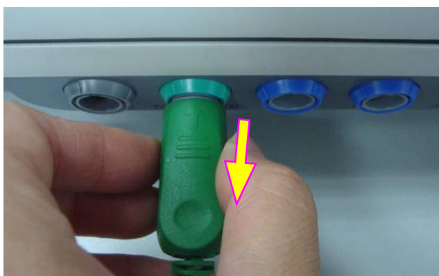
Disconnecting the transducer
