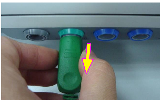
Disconnecting the transducer
