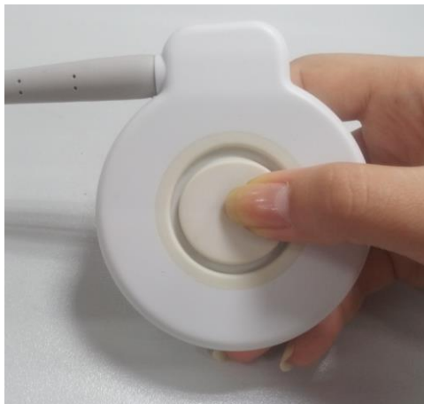
Figure 7-5 Testing a TOCO Transducer
