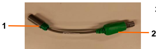
Figure 2-16 IUP Connecting Cable
